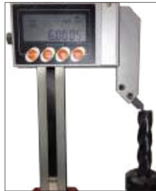
Lock the Z-axis for quick length adjustment
