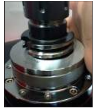
Rotating interchangeable sleeve, with adjustment screws for parallel calibration
