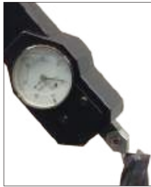
Spring Loaded indicator for reference, with hardened steel tip
