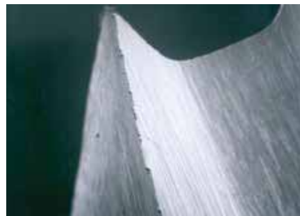
Surface of a conventional fluteless tap
