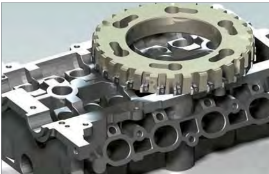
Bottom Face (Roughing & Finishing) - High feed Cutter
