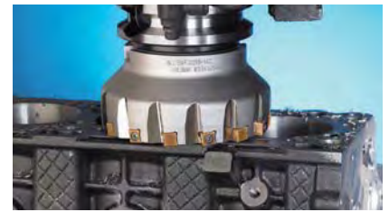
Roughing for cast iron
