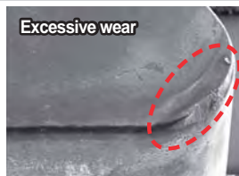
Existing grade (K10)
