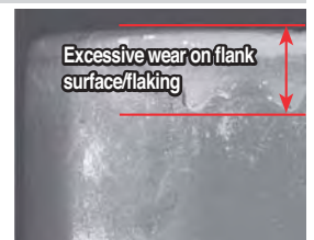
Existing grade (K15)
