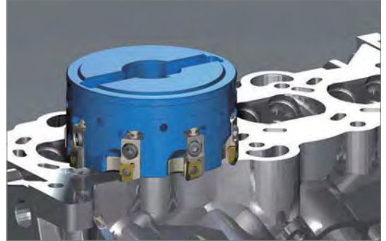
Top Face (Roughing & Finishing) - Aero Mill
