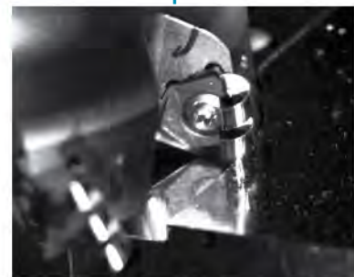
Properly curled chips (The photo was taken by a high speed camera.)
