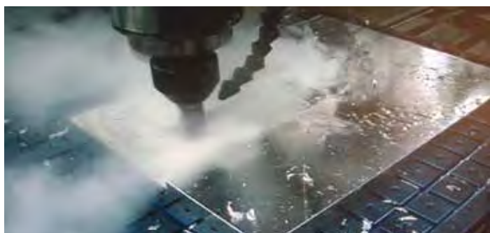
Application using Mitee-Grip™ with sacrificial top plate
