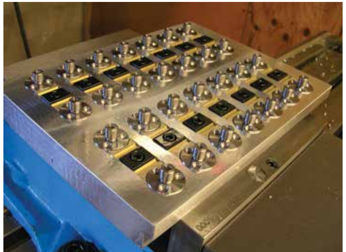
Fixtured with Mitee-Bite Machinable Uniforce® Clamps
