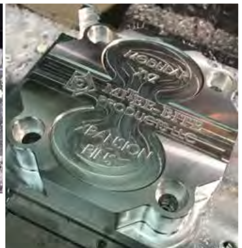
Op 2 including c'bore on same fixture
