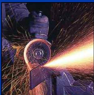
Notching a steel bar prior to welding.
