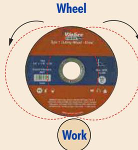
**Counter rotation of the work-piece** is recommended for cutting large cross sections (over 8") and when cutting tubular stock.
