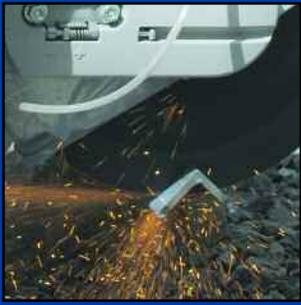
Cutting angle iron with a chop saw.
