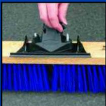
Place handle connector over bolts and tighten lock nuts securely
