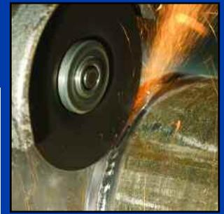
Cutting out weld defects for repair.
