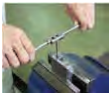
Manual tapping by using tap wrench
