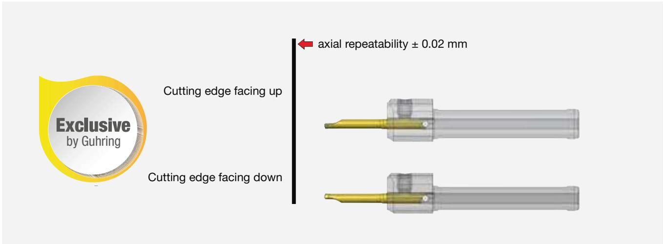
Guhring's system 104/106 is unique in terms of insert positioning and clamping: The position between cutting edge facing up and cutting edge facing down can be changed by keeping the same length position without loosening the holder.
