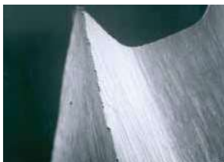
Surface of a conventional fluteless tap
