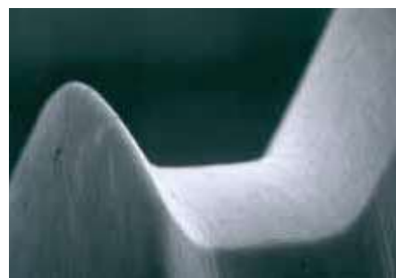
Optimized surface of a Guhring Profile fluteless tap
