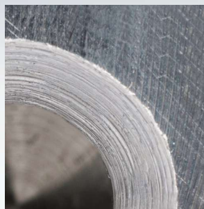
Countersinking with standard countersink
