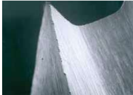
Surface of a conventional fluteless tap
