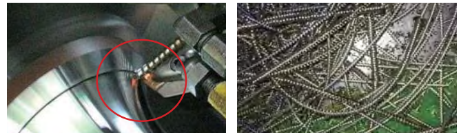
Conventional chip breaker
