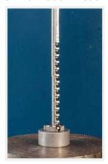
Use of Individual Push-type Keyway Broaches or Keyway Broaches from a Broach Set requires the use of a Bushing and Shim(s). The Bushing size and style are determined by the bore diameter of the workpiece as well as the Style of Broach to be used. "A / I" Style Broaches are used with "A / I" Style Bushings, "B / II" style Broaches with "B / II" Style Bushings, etc. The smallest Broaches cut in one pass and require no Shim. Multiple pass Keyway Broaches
